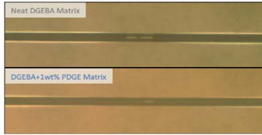
Figure 3: Fiber fractures of unsized, as-received AS4 carbon fiber in single fiber fragmentation test in neat DGEBA and DGEBA + 1 wt% PDGE matrices
