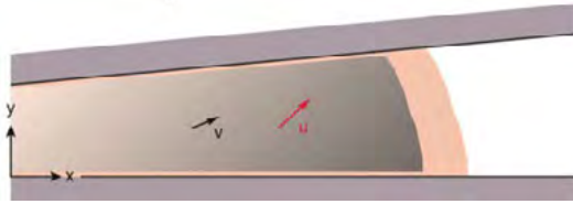
Figure 1: A continuum model of a two phase flow of matrix (red) and fiber phase (grey)
