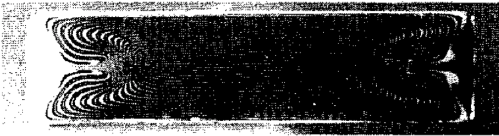
Figure 10 Polystyrene Layer Profile in a Rectangular Channel - 165 Layers
