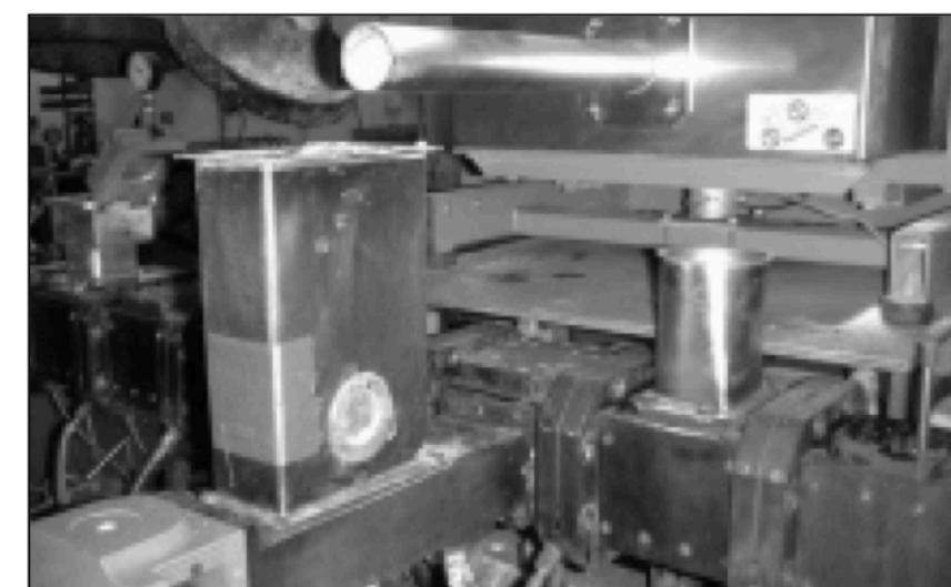
FIGURE 4 Side stuffing of powders
