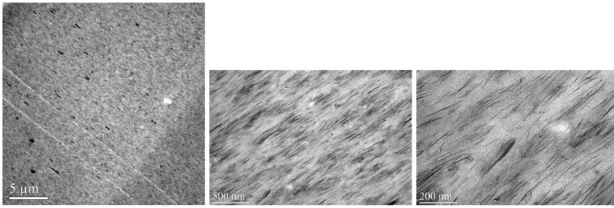
Figure 11. TEM images of zinc ionomer / Cloisite 20A (5 wt. % MMT).
