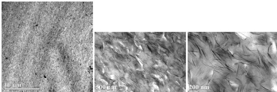
Figure 9. TEM images of sodium ionomer/Cloisite 15A (5 wt. % MMT) composite molded bar (10 lb/hr and 350RPM).
