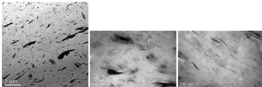
Figure 10. TEM images of sodium ionomer/Cloisite 93A (5 wt. % MMT) composite molded bar (10 lb/hr and 350RPM).
