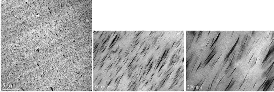
Figure 12. TEM images of zinc ionomer / Cloisite 93A (5 wt. % MMT).
