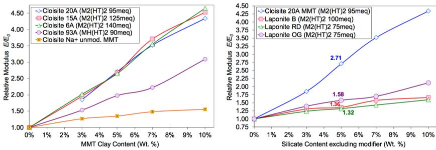
Figure 6. Tensile modulus data for zinc ionomer / layered silicate composites.
