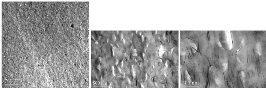
Figure 8. TEM images of sodium ionomer/Cloisite 20A (5 wt. % MMT) composite molded bar (10 lb/hr and 350RPM).
