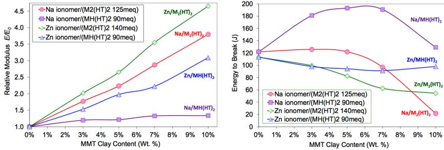
Figure 7. Tensile data comparing zinc and sodium ionomer / Cloisite MMT nanocomposites.
