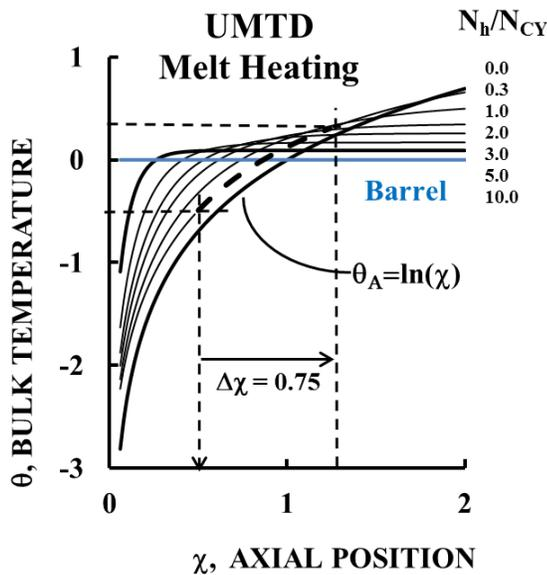
Figure 1. The basic UMTD for Melt Heating. Units are all dimensionless. An adiabatic barrel solution,  $\theta_A$ , is shown as a limiting condition. An example for a single melt zone is shown by the dashed lines.
