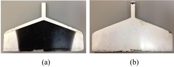
Figure 13. “Frozen” heel from the die with an asymmetrical rectangular manifold geometry similar to the diagram in Figure 4c. The top (a) and bottom (b) surfaces are shown.
