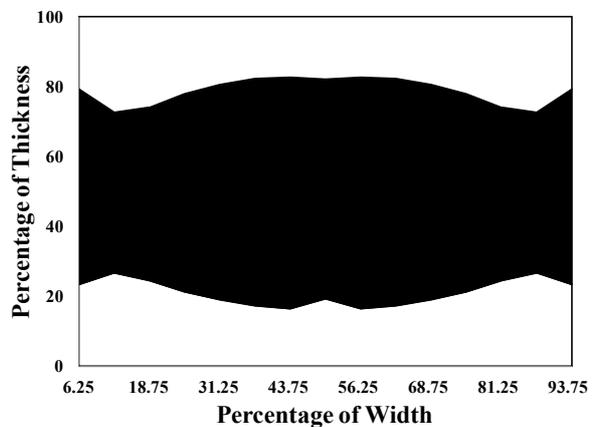
Figure 8. Skin and core layer thicknesses across the width of the die land for a 3 layer structure in a symmetrical manifold.
