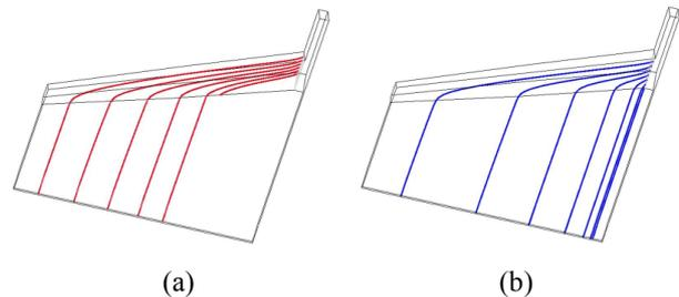
Figure 18. Particle path plots tracing the upper (a) and lower (b) interface locations in a 3 layer structure in a half teardrop asymmetrical manifold.
