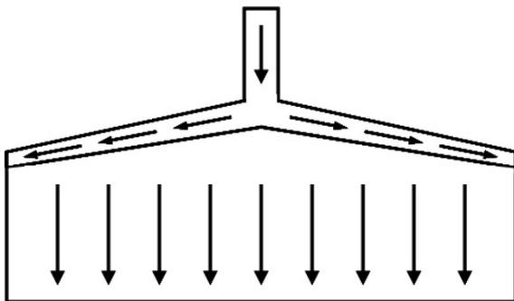
Figure 3. A schematic diagram showing the flow through a coathanger die geometry.
