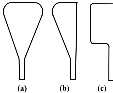
Figure 4. Coathanger die manifold cross-sectional geometries.
