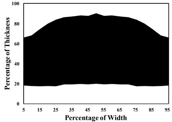
Figure 11. Skin and core layer thicknesses across the width of the die land for a 3 layer structure in a half teardrop asymmetrical manifold.
