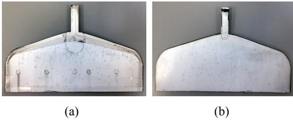
Figure 9. “Frozen” heel from the die with an asymmetrical half teardrop manifold geometry similar to the diagram in Figure 4b. The top (a) and bottom (b) surfaces are shown.
