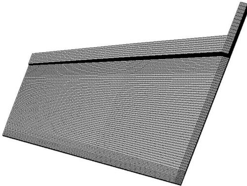
Figure 16. Finite element mesh for a rectangular asymmetrical manifold.
