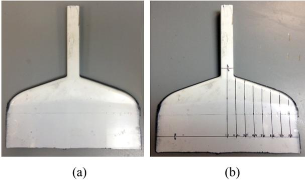
Figure 5. “Frozen” heel from the die with a symmetrical manifold geometry similar to the diagram in Figure 4a. The top (a) and bottom (b) surfaces are shown.
