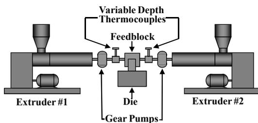
Figure 2. A schematic diagram of the extrusion line.
