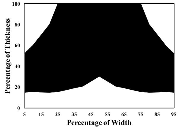
Figure 15. Skin and core layer thicknesses across the width of the die land for a 3 layer structure in a rectangular asymmetrical manifold.
