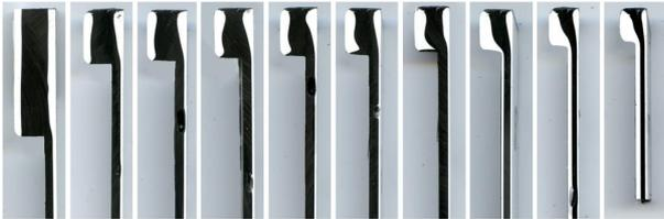
Figure 14. Cross-sectional cuts for a 3 layer structure in a rectangular asymmetric manifold. Flow progresses down the channel from left to right with the image on the left taken from near the center of the die and the image on the right taken from near the edge of the die.
