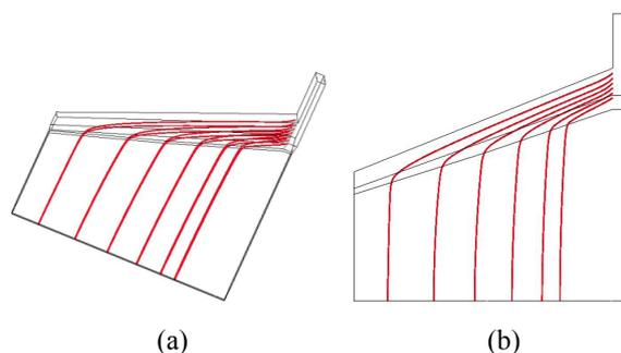
Figure 19. Particle path plots showing the upper and lower interface locations in a 3 layer structure in a symmetrical teardrop manifold, where (a) and (b) show different viewing angles of the final results.
