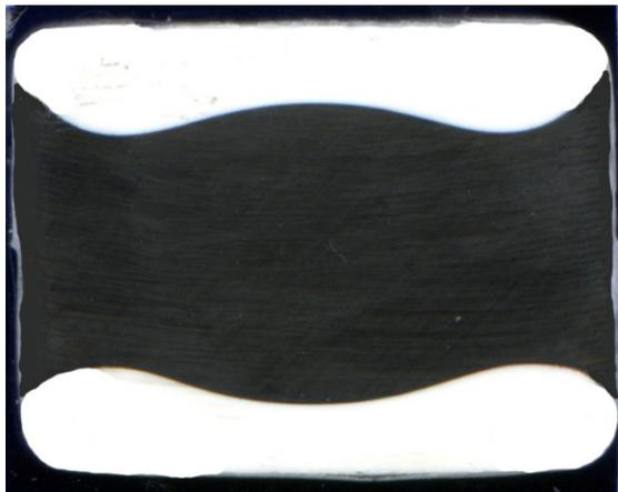
Figure 6. The three layer structure prior to entering the die distribution manifold.
