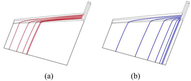
Figure 17. Particle path plots tracing the upper (a) and lower (b) interface locations in a 3 layer structure in a rectangular asymmetrical manifold.
