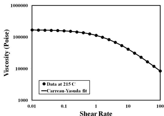
Figure 1. Rheology of HIPS Resin at 215 °C.
