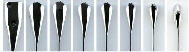
Figure 7. Cross-sectional cuts for a 3 layer structure in a symmetrical manifold. Flow progresses down the channel from left to right with the image on the left taken from near the center of the die and the image on the right taken from near the edge of the die.
