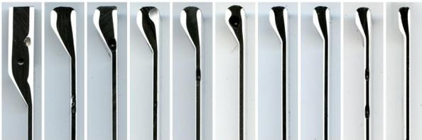
Figure 10. Cross-sectional cuts for a 3 layer structure in a half teardrop asymmetrical manifold. Flow progresses down the channel from left to right with the image on the left taken from near the center of the die and the image on the right taken from near the edge of the die.
