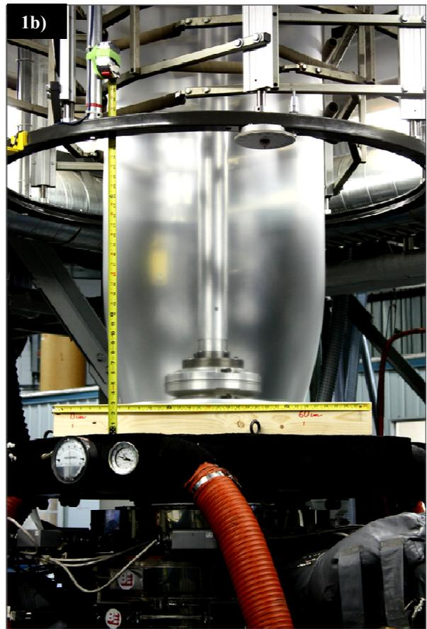
**Figure 1.** Brampton Engineering 9-layer air cooled blown film line. **1a)** Side view. **1b)** Detail view of the 9-layer film formation at multi-layer die exit region including the scale for precise bubble shape determination by using digital image analysis.
