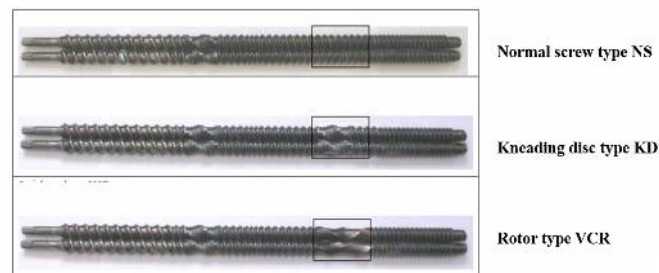
Figure 16. Combination of various mixing screw elements
