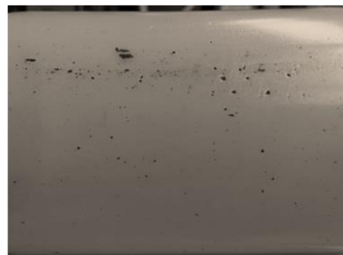
Gels on the surface of a Polyolefin Pipe
