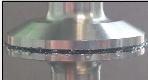
Edge fracture effects in PDMS as a function of the set deformation.
