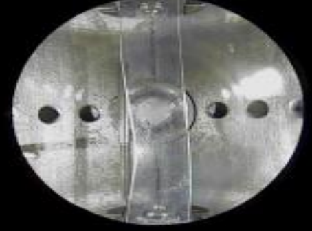
Sagging in a DMA torsion test
