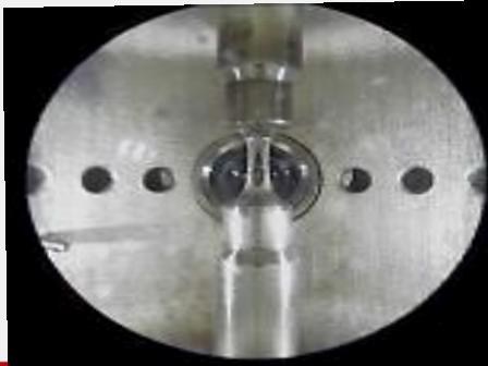
Stringing in a tack test
