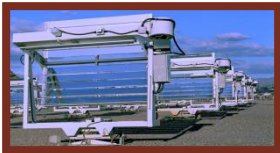
Phoenix, AZ, USA High Desert Benchmark, Accelerated Concentrated Solar Weathering, Atlas Solar Test Center (STC)
