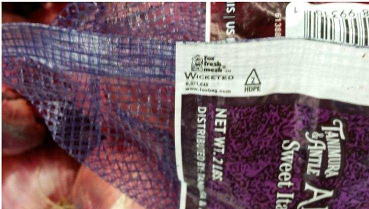
This bag is ostensibly high density polyethylene #2 HDPE. The mesh is #5 polypropylene and the film is low density polyethylene #4 LDPE.
