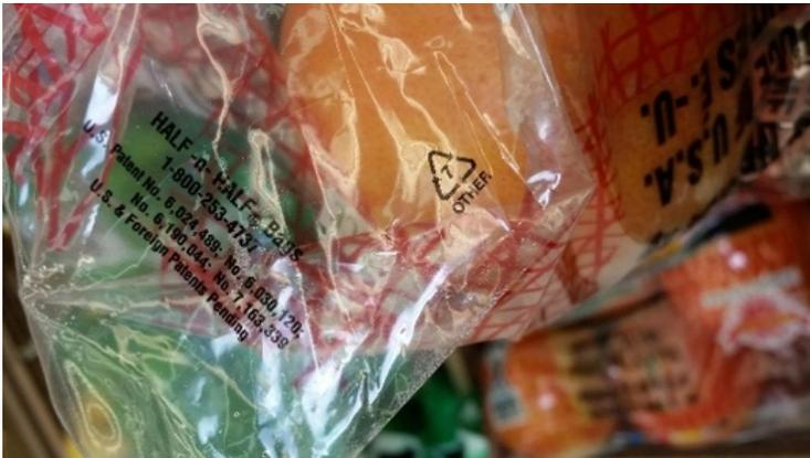
This is an example of a properly executed resin identification code. The RIC #7 indicates the use of 2 dissimilar polymers which make it a #7
