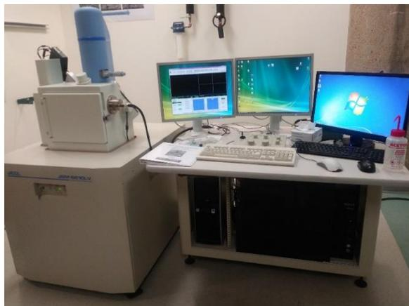
Fig. 8. JEOL JSM-6610LV Scanning Electron Microscope
