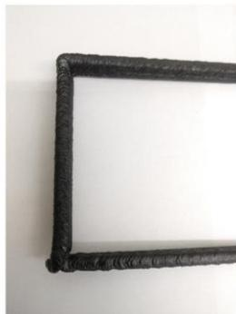
Fig. 2. Test specimen with 13% weight fraction carbon fiber ABS
