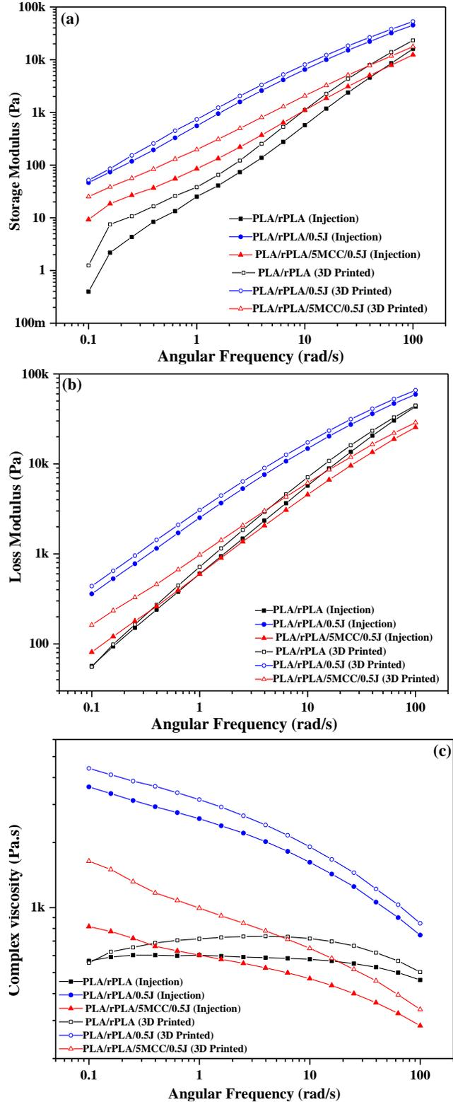
Figure 3: Rheological properties of PLA/rPLA-based samples; frequency vs: (a) storage, (b) loss modulus and (c) complex viscosity.
