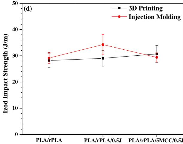
Figure 2: (a) Tensile modulus, (b) tensile strength, (c) %elongation at break and (d) Izod impact strength of injection and 3D printed samples.
