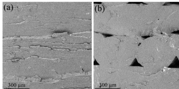
Figure 1: Surface topography of (a) and (b) PLA/rPLA/5MCC/0.5J, developed using injection molding and 3D printing, respectively.
