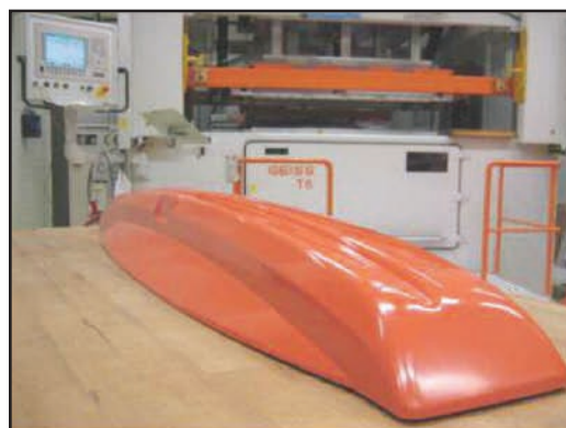
Figure 4. A big part formed from a non-FR PC / PBT formulation with 12% thermoforming additive (1390 x 280 x 135 mm 3 ).
