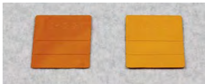
FIGURE 5: Two different results from one color concentrate molded at two different temperatures.
