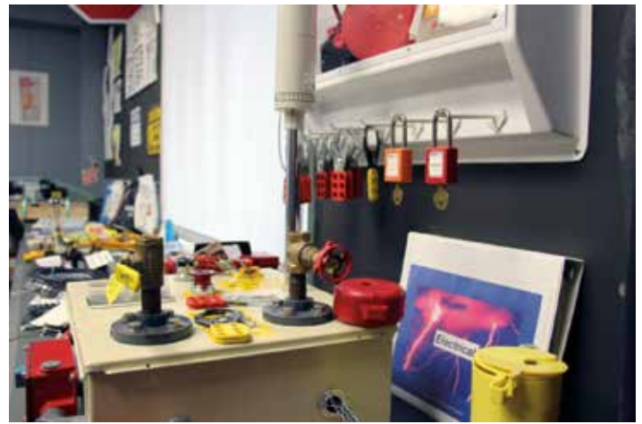
FIGURE 2: Lock out tag out. One of the 26 workstations in the Dojo
