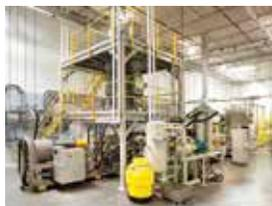
Mezzanine mounted LIW feeders provide precision controlled feed blends and instantaneous formulation changes
