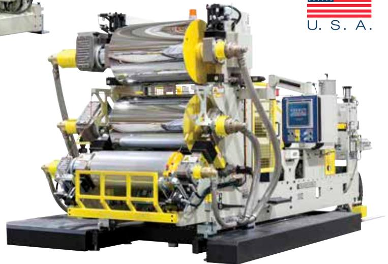
G-Series® Configurable J-Stack roll stands offer unique processing benefits, including higher output capability for medium through heavy gauges when running lower melt strength resins. Additionally, PTi's G-Series® roll stands offer more advanced features and technical solutions for sheet production than any others.
