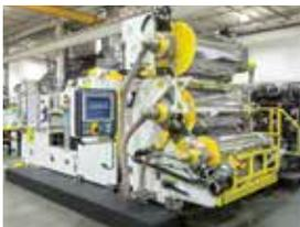
G-Series® Configurable J-Stack features individual roll drives, hydraulic actuation, safety roll lock-out, guarding, trip chords and e-stops, & TITAN® PLC pendant
