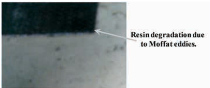
Figure 6. Photograph of resin degradation at the flight radii due to long residence time in the region by Moffat eddies.
