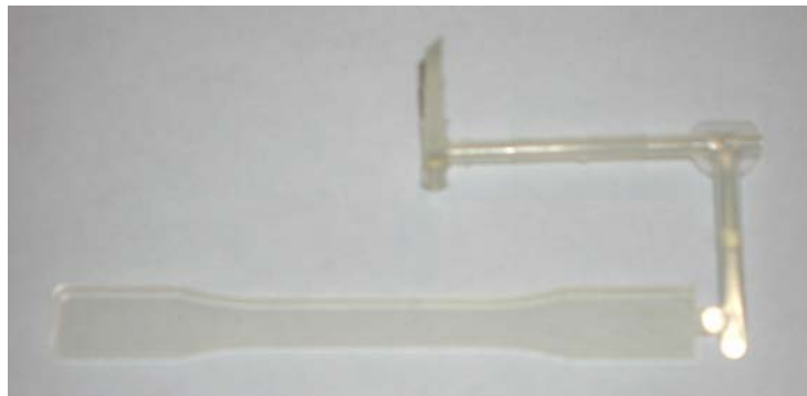
Figure 1. Runner layout and specimen
