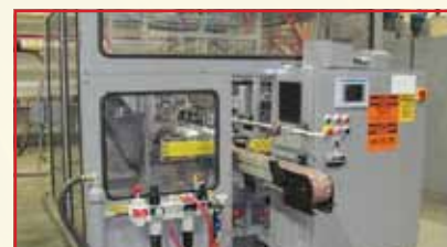
Close-up of controlled scrap release system R&B 4-Bottle Deflash Trimmer with and container specific deflash tooling
