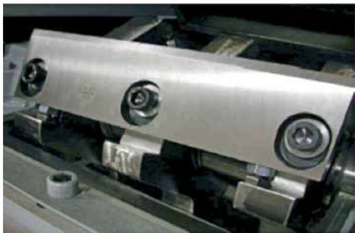
Figure 15a. Checks to be sure that proper knife tip angle is maintained.
