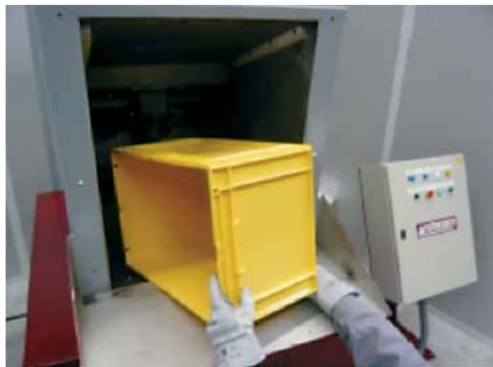
Figure 17b. Large part pre-size reduction can be accomplished with augers.
