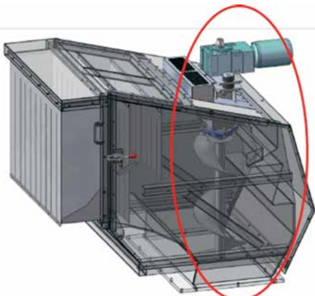
Figure 18. Auger screw allows for smaller granulator with smaller cutting circle to be used.
