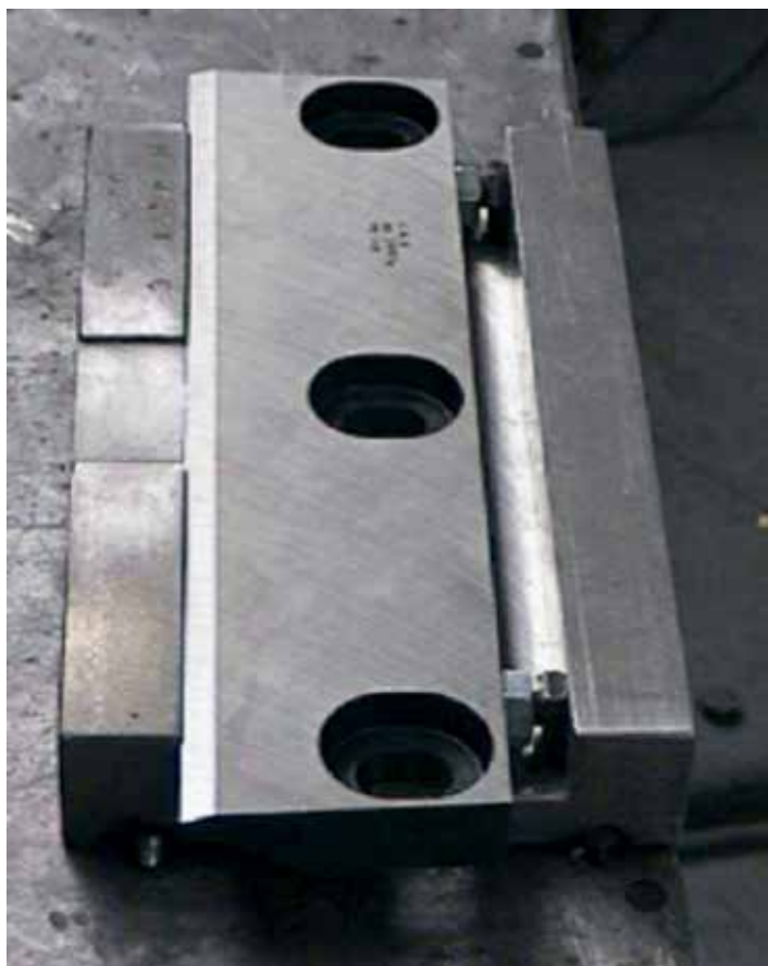
Figure 15b. Knife gap pre-adjustment fixture allows for knives to be gapped outside of the machine.
