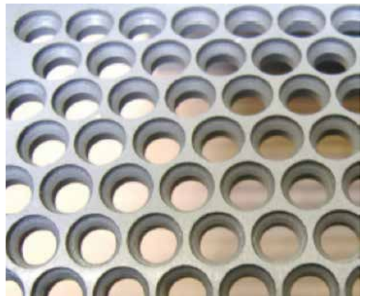
Figure 14. Close-up view of conical hole design in screen.
