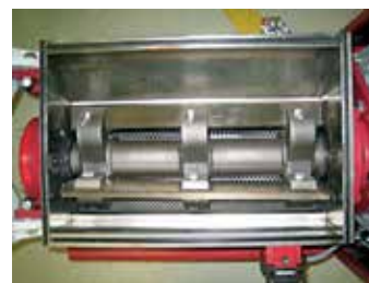
Figure 5. Open rotors take bigger bites and allow for the most air flow through the cutting chamber.
