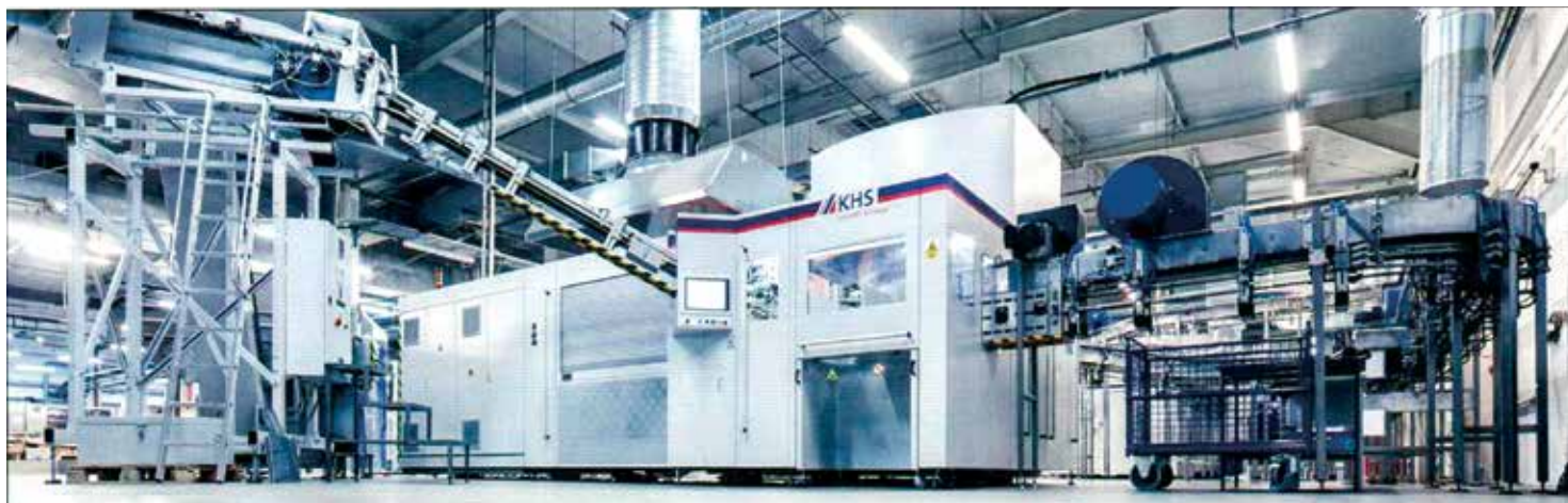
Below: A present-day KH InnoPET Biomax Series IV stretch blow moulder reached outputs of more than 60,000 bottles per hour.
