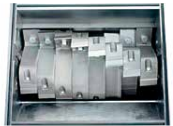
Figure 6. A staggered style rotor is designed to nipple on thick cross-sectioned feedstock like flash, but restrict air flow.
