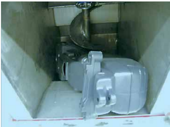
Figure 17c. Large part pre-size reduction can be accomplished with augers.
