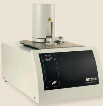
**Differential Scanning Calorimetry (DSC)** to investigate glass transition and melting behavior
