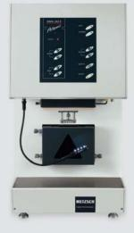
**Dynamic Mechanical Analysis** (DMA) to characterize stiffness and damping behavior
