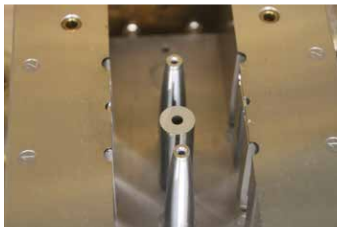
Special feature: the plastic is injected into the mold from the ejection side. This has proved to be the most efficient design for these injection moldings.
