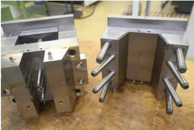
Clear to see: the guides for the angle pins at the base of the splits. This reliably protects against lining up and tilting during operation.
