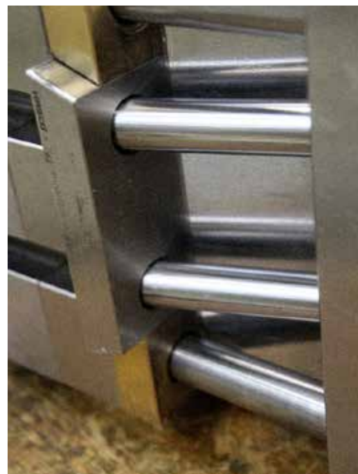
The angle pins reliably in their guides. The HASCO mold bases have already proved successful in many projects at Bruno Eugster.
