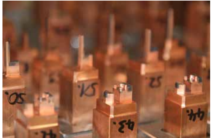
Eugster generally performs erosion with copper electrodes, as most workpieces require a high surface quality.
