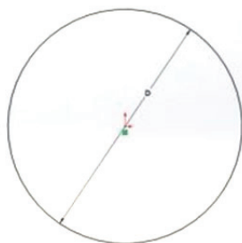
Figure 2. The hydraulic diameter of a round passage is equal to the hole's diameter.
