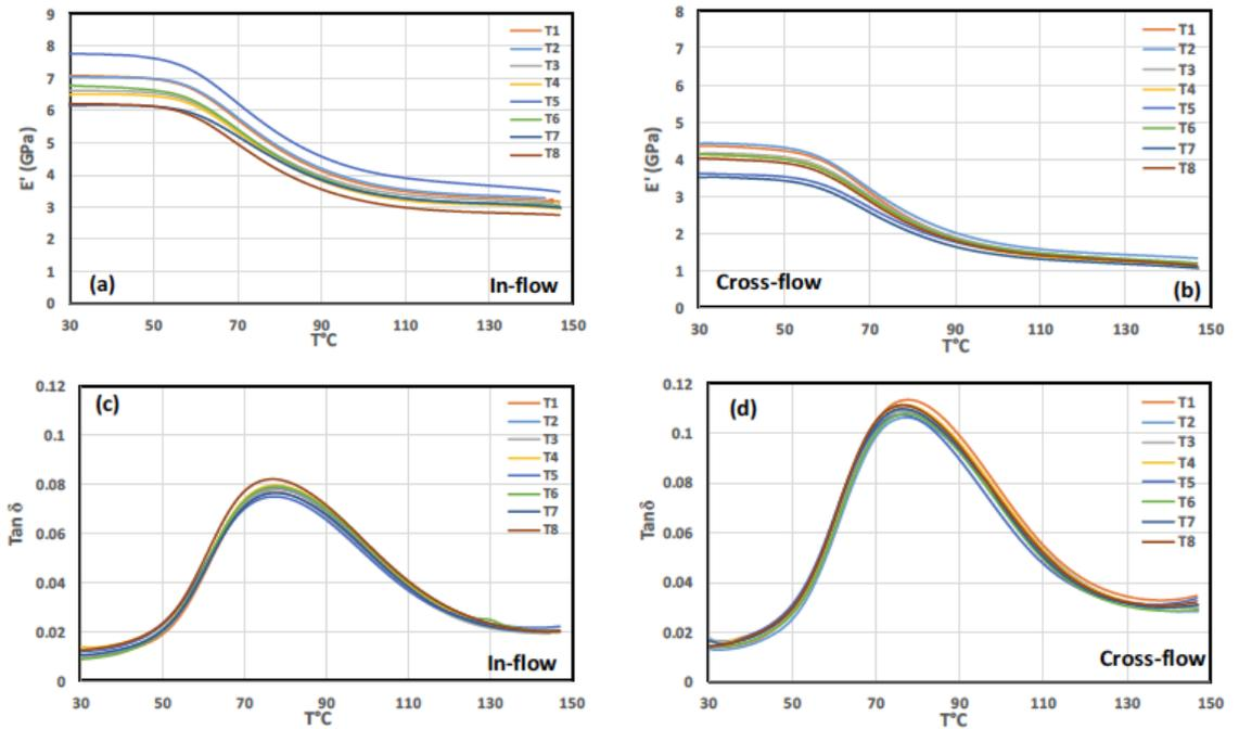
Figure 4 Storage modulus as a function of temperature with the change of processing parameters
