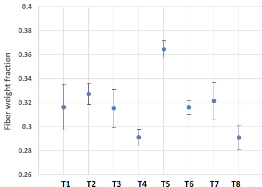
Figure 9 Fiber content obtained by burn-off test for plaques with different processing parameters
