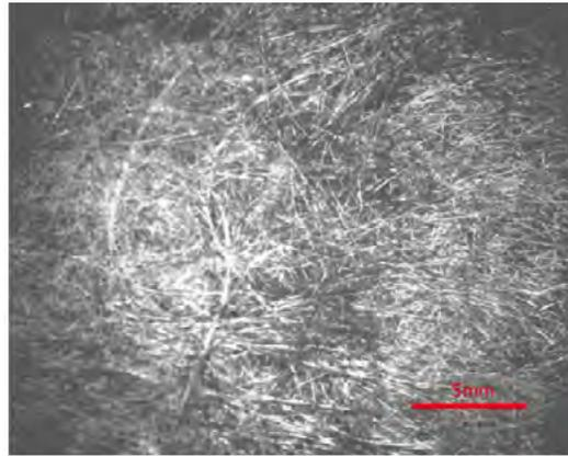
Figure 10 Optical microstructure of GF after PA6 burnt-off (to be replaced if a better one obtained)
