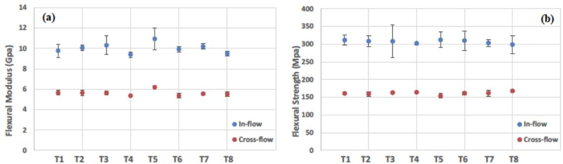
Figure 6 Comparison of the effects of processing parameters on flexural properties (a) Flexural modulus; (b) Flexural strength
