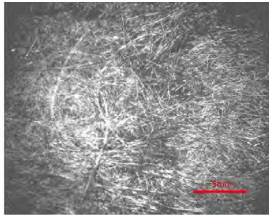
Figure 10 Optical microstructure of GF after PA6 burnt-off (to be replaced if a better one obtained)
