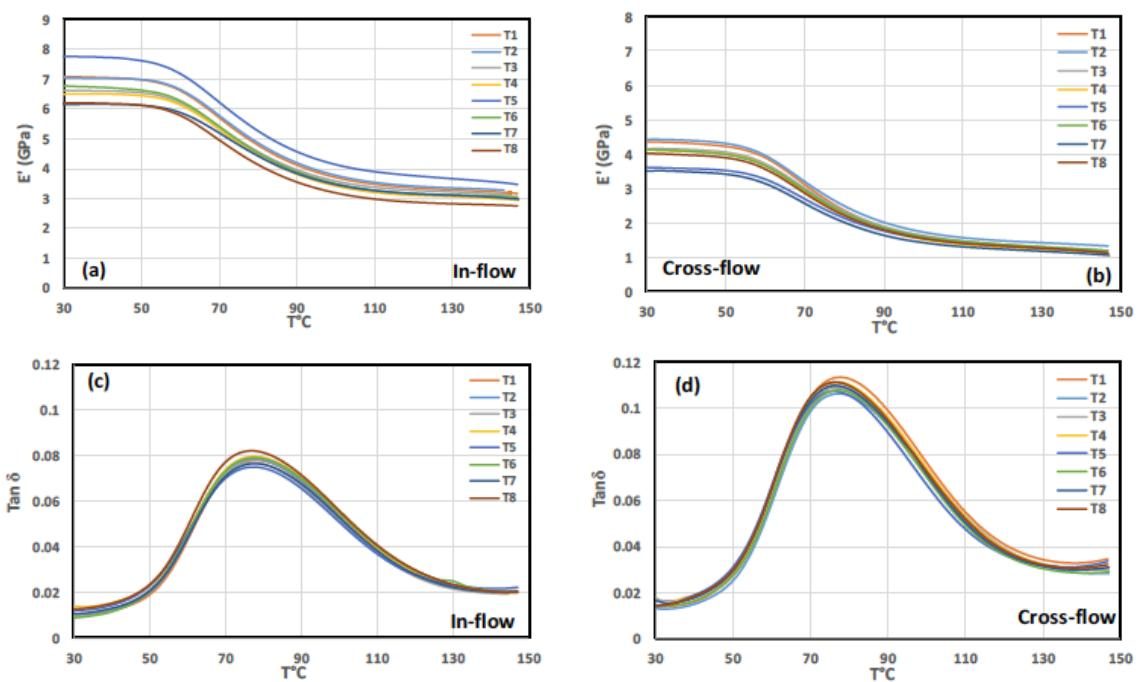
Figure 4 Storage modulus as a function of temperature with the change of processing parameters
