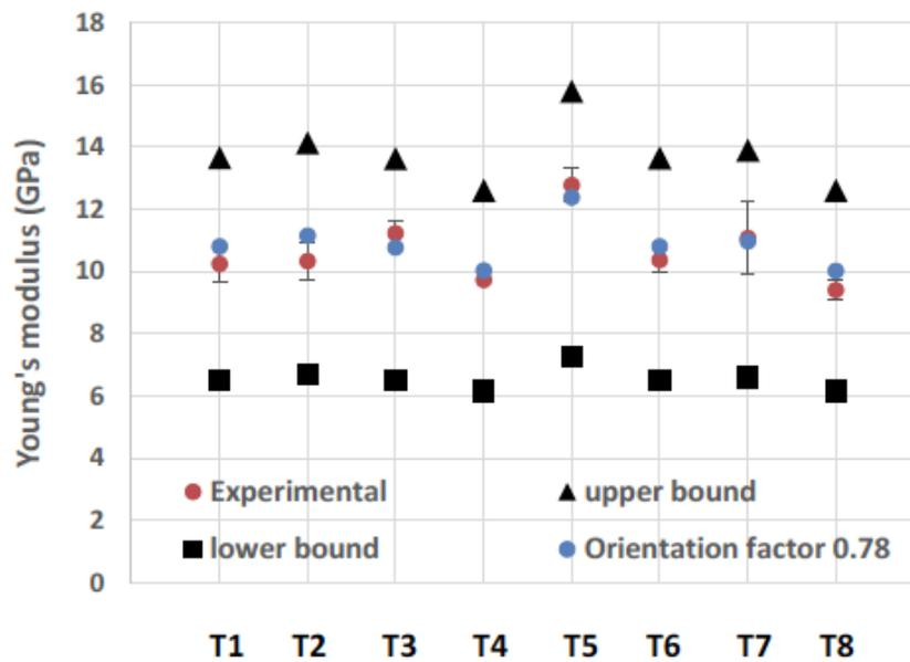
Figure 11 Comparison of experimental Young's modulus with the predicts of upper (unidirectional) and lower (random) bound and orientation factor of 0.78
