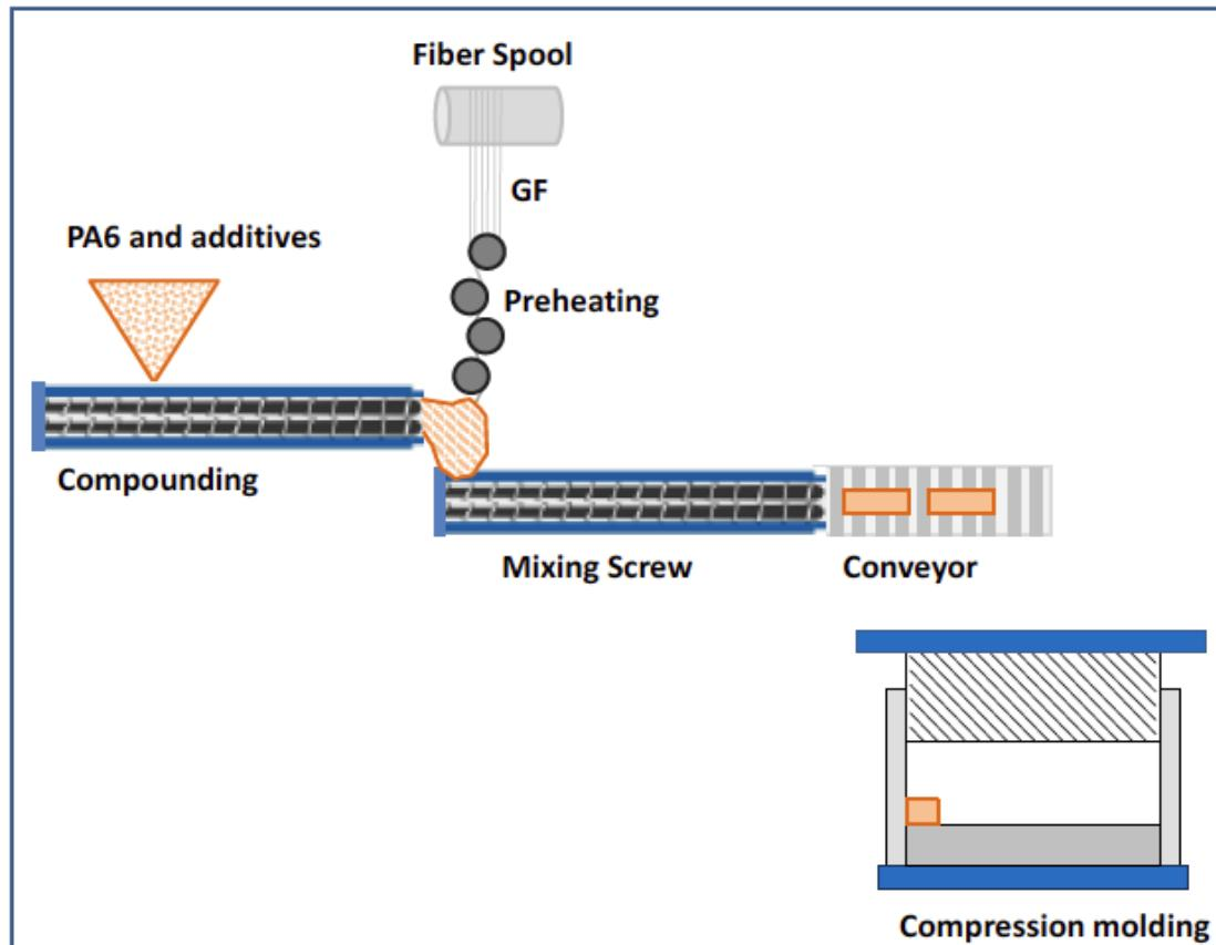
Figure 1. Diagram showing the LFT-D-ECM line used for producing plaques
