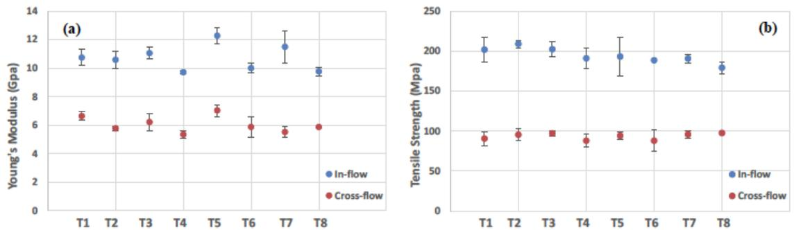
Figure 5 Comparison of the effects of processing parameters on tensile properties: (a) Young's modulus; (b) Tensile strength
