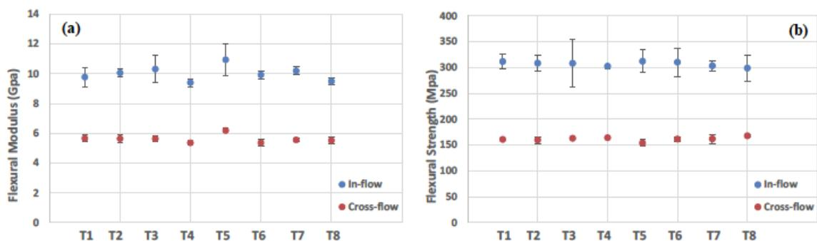
Figure 6 Comparison of the effects of processing parameters on flexural properties:
