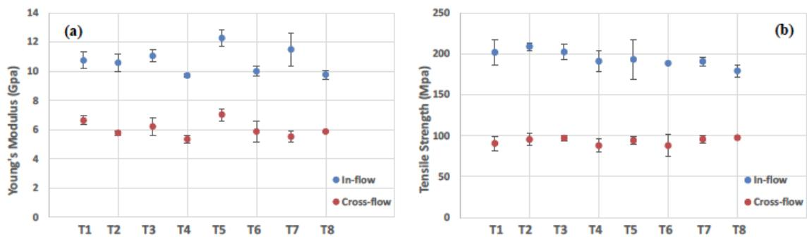
Figure 5 Comparison of the effects of processing parameters on tensile properties:
