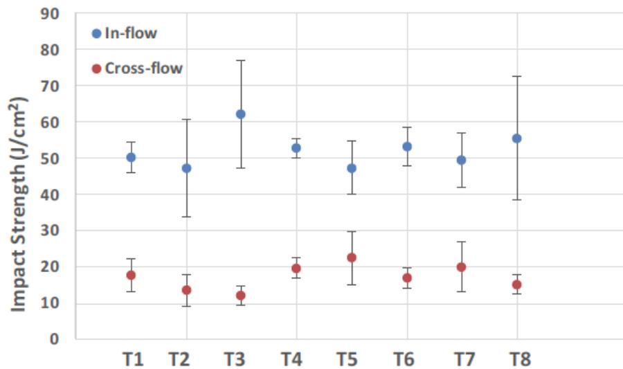
Figure 7 Comparison of the effects of processing parameters on impact strength
