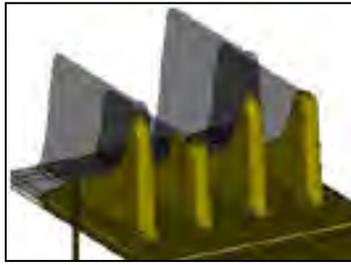
Figure 18: Flow front inside the straight rib section in simulation
