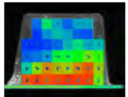
Figure 17: CT analysis of fiber content showing significant change in fiber content in straight rib
