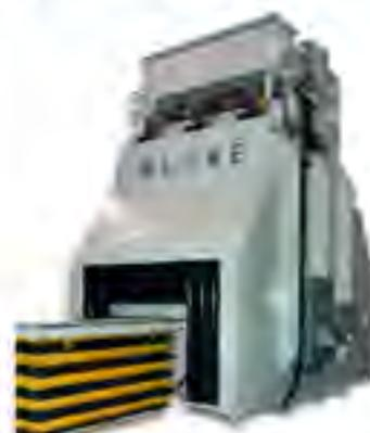
**Typical Autoclave Batch Cure: 4-6 Parts (180 - 360 minute cycle)**
