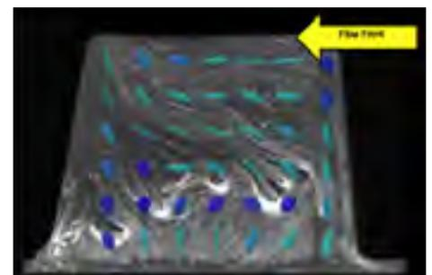
Figure 21: Fiber orientation in CT analysis of straight rib (side view)
