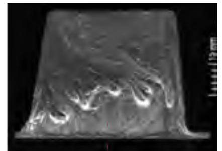
Figure 16: CT image of the straight rib showing excessive fiber bundling and change in fiber content
