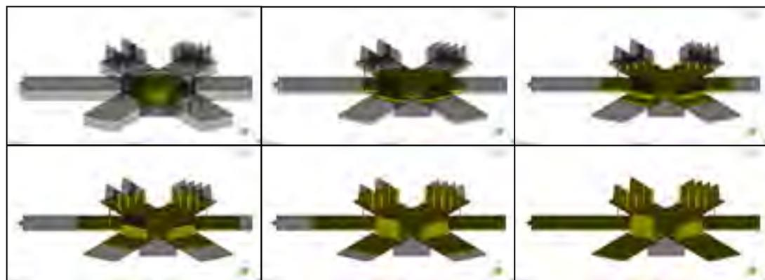
Figure 4: Mold filling simulation in compression molding at different time steps
