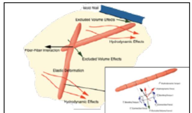
Figure 29: Direct Fiber Simulation with a micromechanistic model [11]
