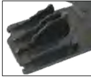
Figure 19: Flow front during straight rib filling in experiments
