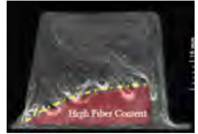
Figure 20: Border region between high fiber content and low fiber content in a straight rib
