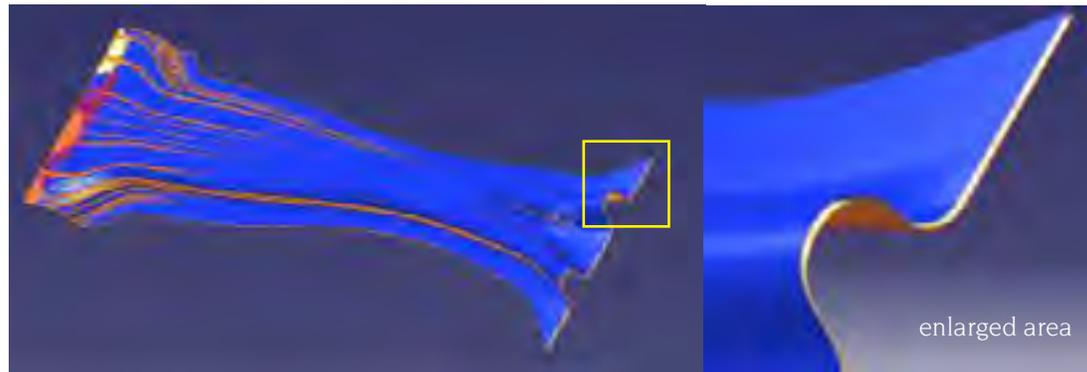
Figure 11: Geometry compensation using Composites Link and CATIA.
