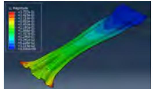
Figure 10: The as-designed part underpredicts deformation by almost 20 percent.
