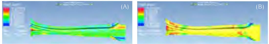
Figure 6: Shear angles for the pressed preform in the (a) top layer (0/90) and (b) second layer (45/-45).
