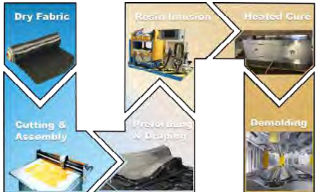
Figure 1: HP-RTM process flow diagram.
