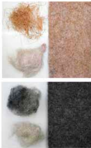
Figure 5. Comparison of tufts of coir (fiber) and propylene fiber (top) and tufts of PET and PE binder fiber (bottom). These are carded and needle punched for felt used to compression mold into trim parts.
