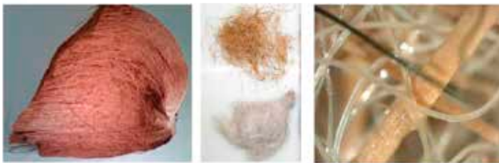
Figure 6. Inside of coconut husk, tufts of coir fiber from husk and PP binder fiber, seen in scanning electron microscope (SEM) after being carded and needle punched.
