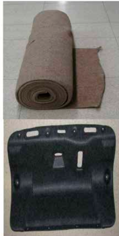
Figure 7. (top) Tufts of coir fiber and PP made into a felt 2-meter wide by 30 meters long. (bottom) PP+PET felted and compression molded into a trunk lid cover.
