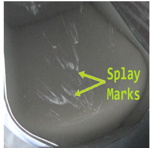
Fig. 1: Splay marks on a molded part
