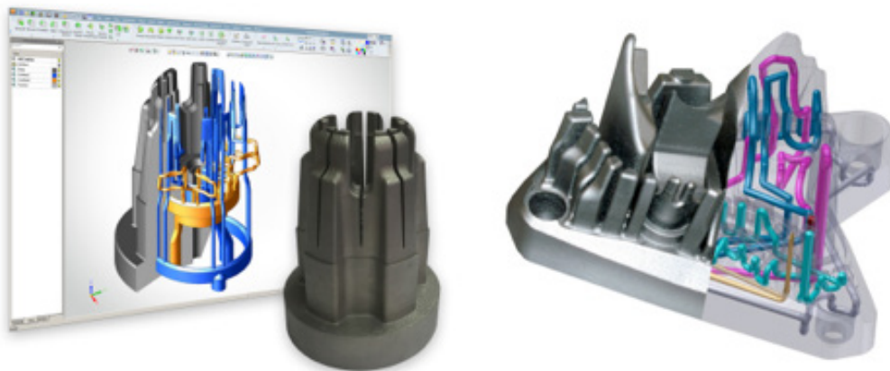
State-of-the-art conformal cooling channels like these from 3D Systems and Renishaw show round channels like traditional drilled cooling lines. But round may not be the most efficient shape. Triangle, star and X-shaped channels all have more surface area and cool better. Left photo: 3D Systems; Right photo: Renishaw;
