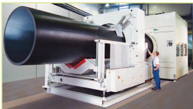
A battenfeld-cincinnati pipe-extrusion line. The company reportedly has developed more efficient single- and twin-screw extruders that are able to melt various materials at lower temperatures than previously possible (photo courtesy of the company).
