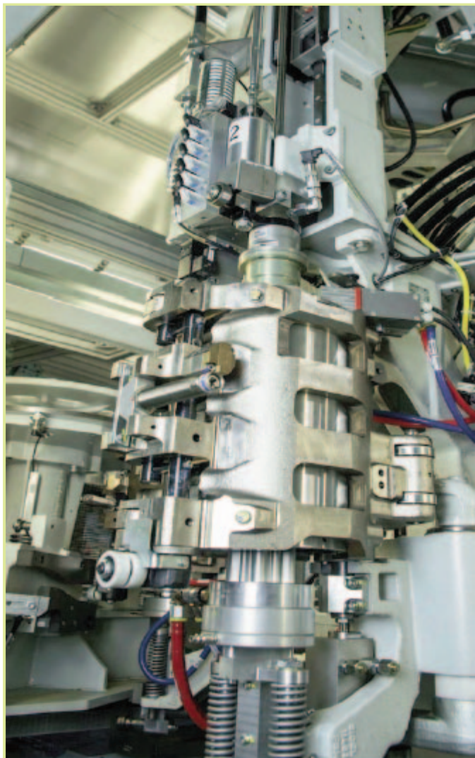
Sidel's Matrix™ blower eHR system uses electrical heating rather than traditional hot oil in bottle blow molding, creating an energy savings of up to 45% (photo courtesy of Sidel).
