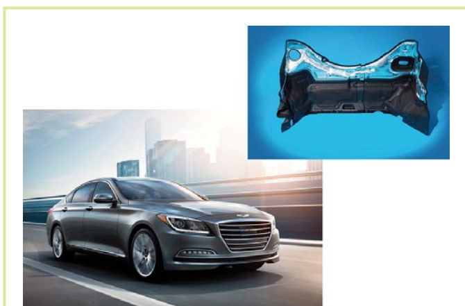
Injection molded long-glass PA 6/6 and barium sulfate have replaced stamped and painted steel for an engine-compartment partition wall on 2015 Hyundai Genesis luxury sedans. The composite partition wall reduced mass by 20%, and improved sound damping by 8 dB while also reducing part count and assembly time, and eliminating paint. (Part photo courtesy of SPE Automotive Division; vehicle photo courtesy of Hyundai Motor Group.)
