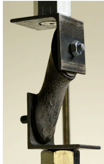
Figure 16. Transmission mount during shear test.
