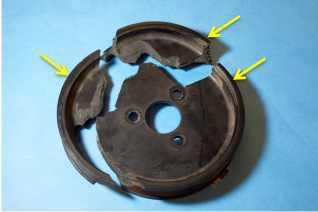
Figure 1. Subject power steering pump pulley. Witness marks indicated.
