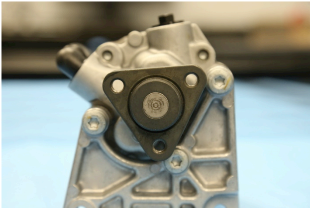
Figure 2. Power steering pump with triangular mounting plate (pulley not installed).
