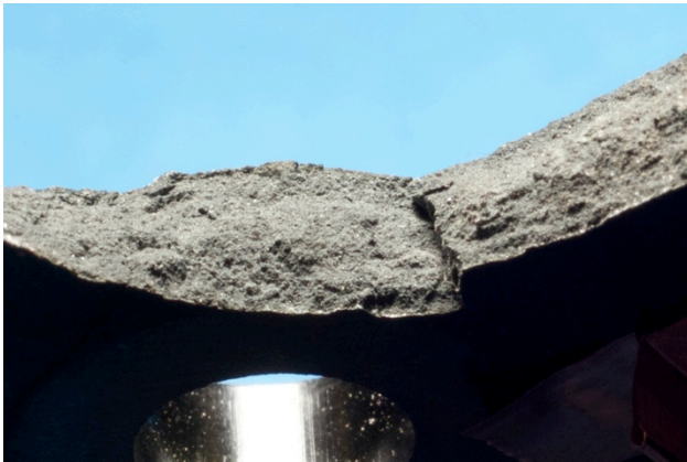
Figure 3. Fracture surface of subject pulley near the likely origin.
